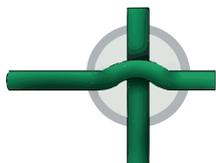
Pipeline cross overs should be made with the use of components specially designed for this purpose.
