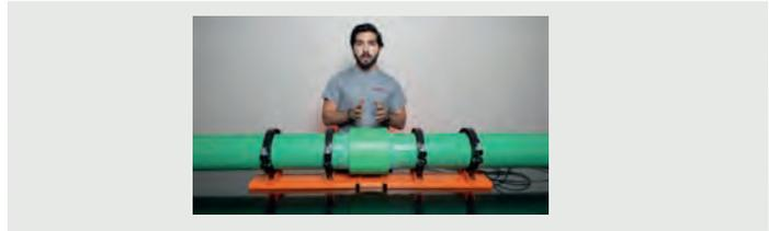
**2.7** Removed the waterproof safety cap, insert the copper head of the welding machine.
