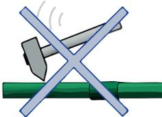
Components of plastic piping system must be protected against damage during transport and installation.
