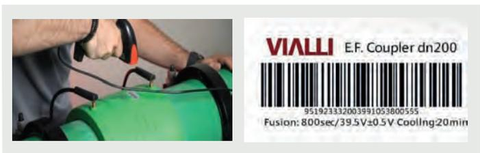
**3.2.3** Finish setting parameter, press ESC button go to main menu, press welding button to check the parameter correctly, finally press OK to start fusion.
