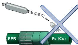
Brazing or soldering of metal fittings should not take place close to the joint between metal plastic systems because of the potential hazard of heat transfer to the fitting.
