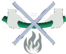
Components must not be exposed to naked flames.
