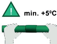
A minimum temperature level for plastic piping installation is with regard to welding, +5°C. At lower temperatures it is difficult to provide working conditions for high quality pipe joints.
