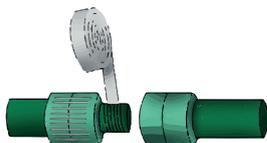
Threaded fittings must be used for screw type joints. Threads should never be cut directly into plastic components. Threads are sealed with a special PTFE tape or sealing compound.
