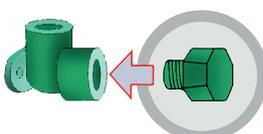
It is recommended to use plastic plugs for blanking elbows or wall mounting groups (plastic plugs are designated only for temporary use). For long-term blanking has to be plugged with metal thread.
